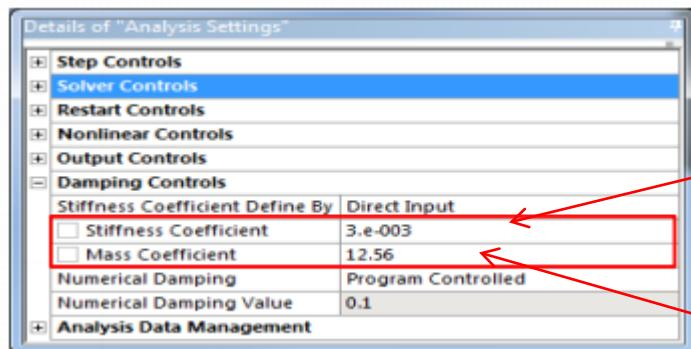
$$\alpha = \frac{2\xi\omega_1\omega_2}{\omega_1 + \omega_2}; \quad \beta = \frac{2\xi}{\omega_1 + \omega_2}$$
